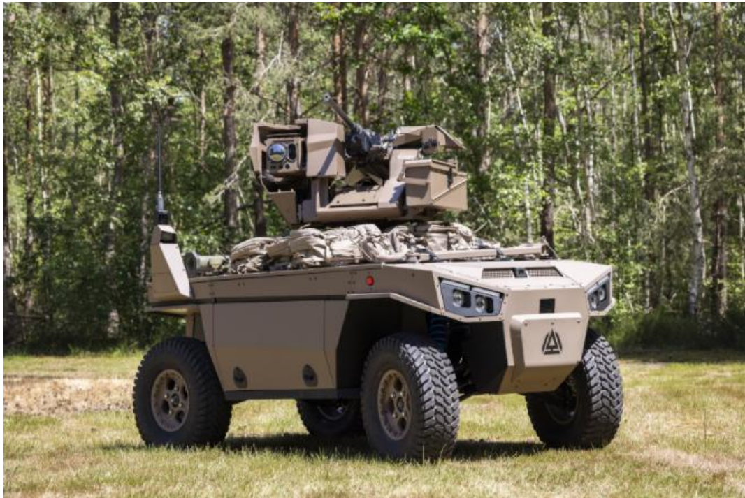
DRAILER platform equipped with an integrated HORNET T1 Remote Weapon Station.
